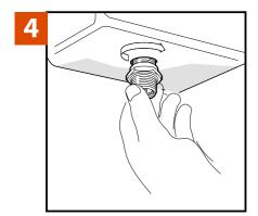
Thread the Femco Drain plug in by hand until snug against the pan. If you meet resistance, back the plug out and try again. DO NOT FORCE the plug into the hole.
