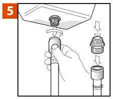
Detach the drainer by unscrewing it from the Femco Drain plug. The valve will return to the "closed" position.
