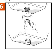
Screw the dust cap back on to the Femco drain plug (by hand)
