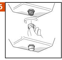
Screw the dust cap back on to the Femco drain plug (by hand).
