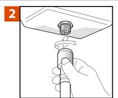
Thread the drainer on to the bottom of the Femco drain plug.
