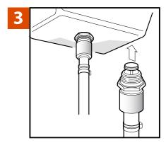
When the drainer is attached to the Femco drain plug, the valve will remain in the open position.
