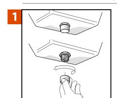
Warm up the engine to operating temperature. Turn off engine. Remove the dust cap from the Femco drain plug.
