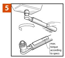
Use a Torque Wrench to tighten the Femco drain plug to the specifications on the container. DO NOT install without using a torque wrench.
